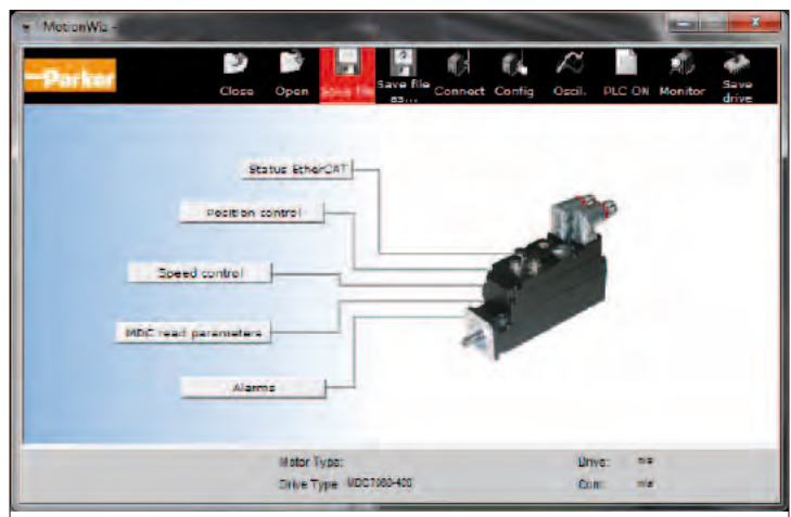
MotionWiz: MDC page - Main electronic control parameters and fieldbus status
